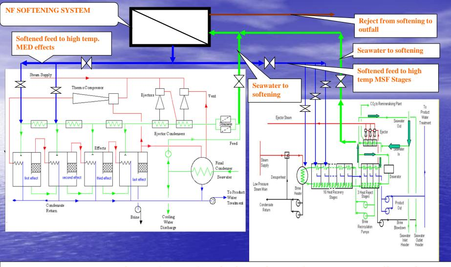
Process and apparatus for partial blending of softened feed to high temperature effects of MED and/or high temperature stages of MSF, in order to increase TBT and Flow of Recycle or Feed
